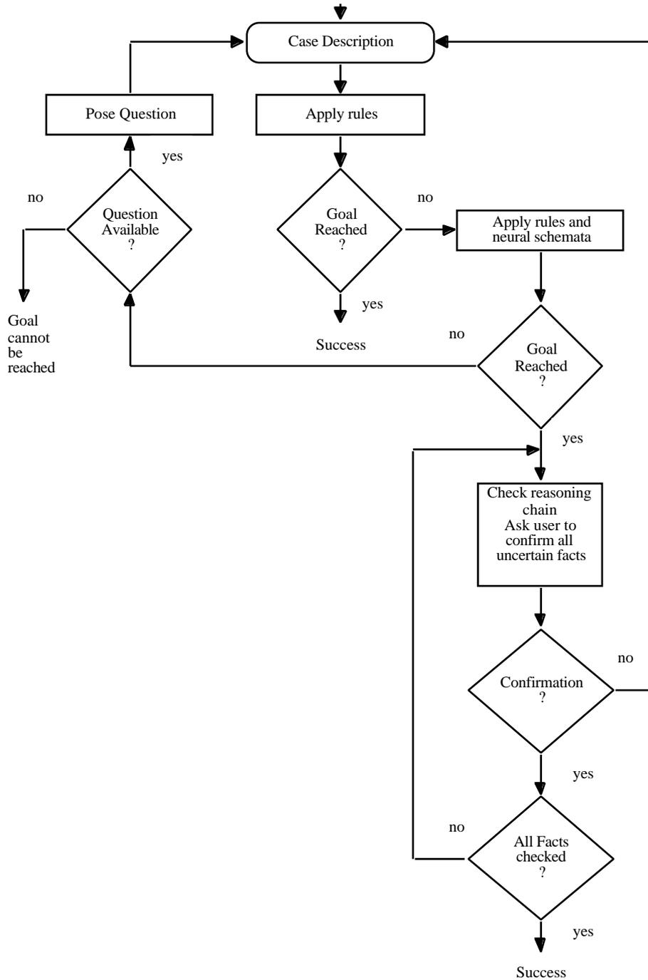
Figure 2: Control strategy to integrate neural schemata in a rule based system
